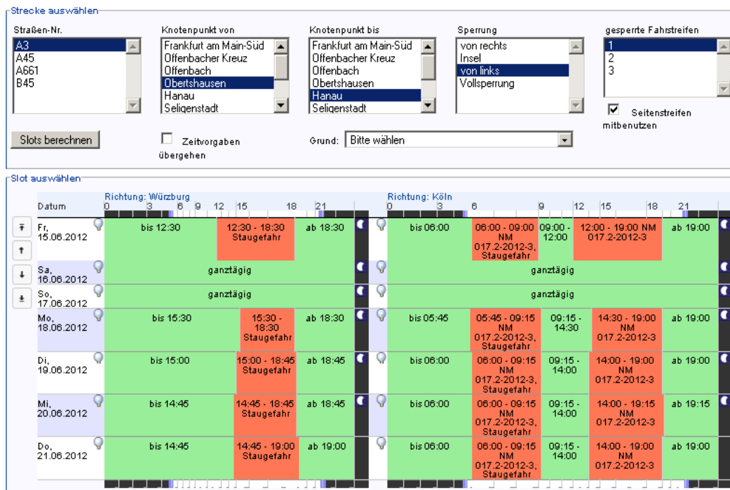
Figure 11.1: Slot management system (source: Hessen Mobil)
