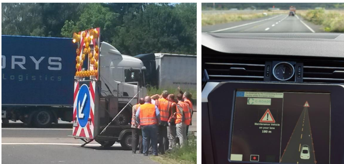
Figure 14.2: Left: Sharing real-world C-ITS pilot experience in Hessen. Right: In-vehicle view of the C-ITS service Maintenance Vehicle Warning of the C-Roads pilot Hessen.
