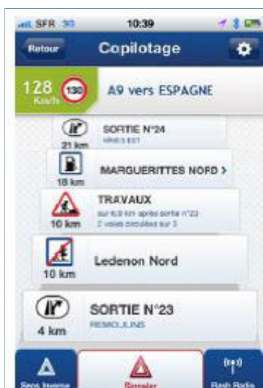
Figure 3 – Screenshot of the virtual VMS board presenting roadworks at 10km after an exit and a rest area closure
