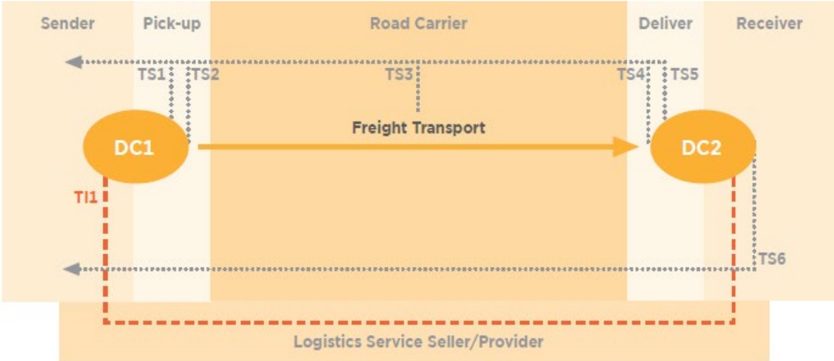
Figure 17. Typical TI and TS message exchanges involved for a single freight consignment; GS1 Australia, 2020 - Freight Data Exchange Pilot Project - Summary Report
