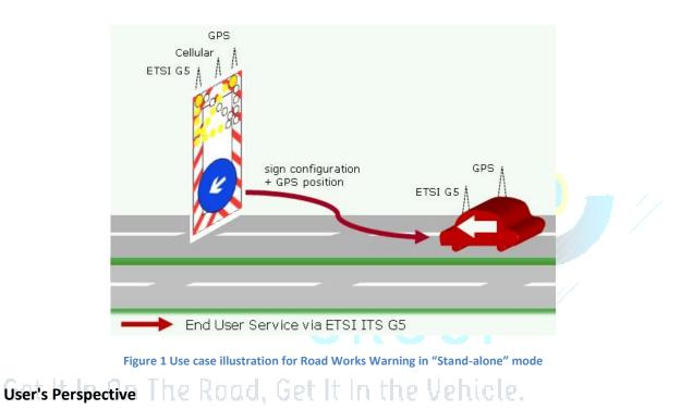
The driver approaches a stationary or mobile road works site. The driver's vehicle HMI presents a warning to the driver. The information provided complies to the functional, operational and technical requirements as specified.
