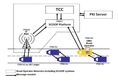
The Scoop ITSS-C, named Scoop Platform, is an ITSS that can be deployed at any TCC of any road operator. It is used by the 5 pilot sites involved in Scoop, in various environments. It aims at storing, processing and communicating (in real time) data from the TCC the vehicles via RSU and/or road operators' OBU (OBU-ro) and vice versa. Datex II standards are used (CEN TS16 157/1-6).
