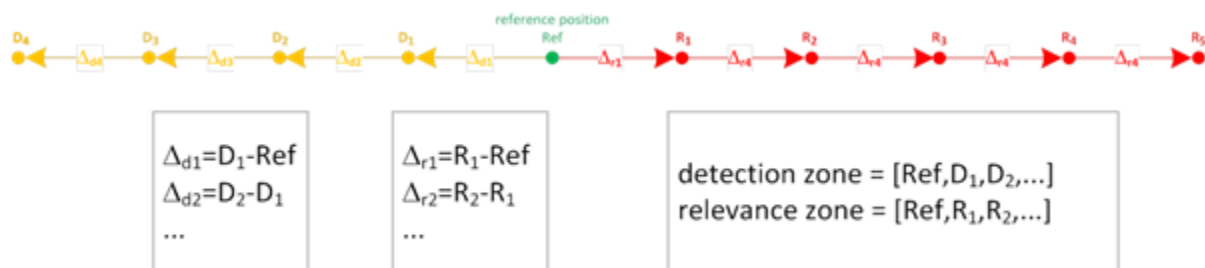
Figure 27: Calculation of DeltaPositions for relevance zone and detection zone respectively
