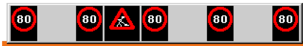
Figure 15: Output of the CORBA test system, visualizing a VMS gantry on A23
