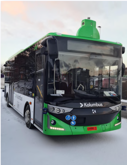
Figure 5: Full-sized automated bus pilot 14
